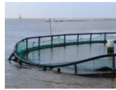
This cage's handrail tube collapses.
